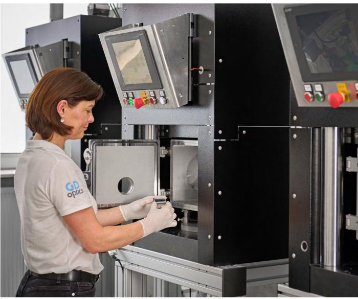
The isothermal process can be used to produce a large number of finished lenses that do not need to be machined afterwards. With its unique know-how in tool making, GD Optics can use the isothermal molding process to produce A-cylinder lenses, aspheres and spheres in a very wide range and in the highest quality. This includes particularly small microlenses with focal lengths  $\ge 250 \ \mu m$ .
